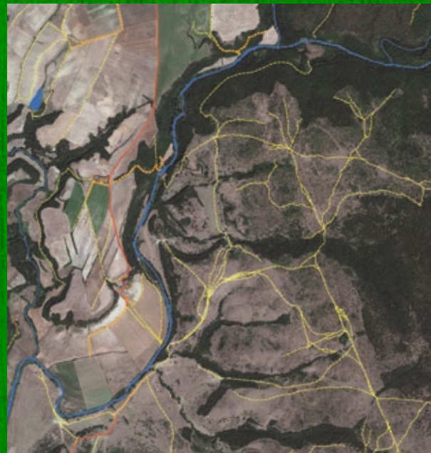
Vector extraction allows roads, hydrology and other features to be mapped using satellite imagery.
