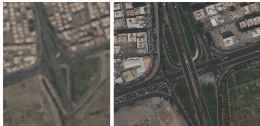
Five-meter imagery (left) can be ideal for mapping larger areas, but it won't show the same level of detail as high-resolution imagery (right).
