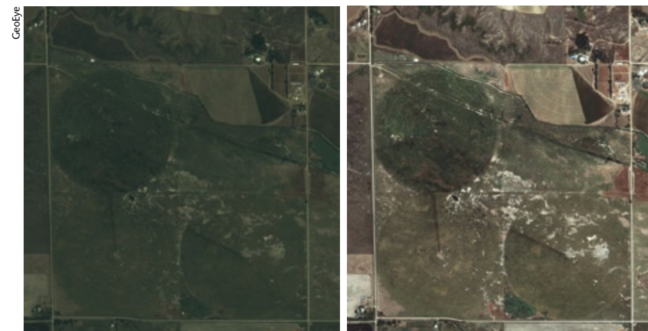
Whether DRA is off (left) or on (right) dramatically affects an image's visual interpretability.
